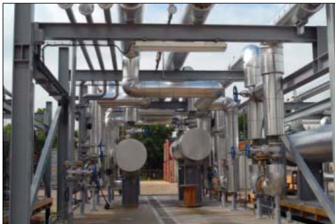
The crude/diesel pump around exchanger module, left, and crude unit pump module await shipment to northern Iraq at the Pasadena, Tex., yard of Ventech Engineers Inc.
