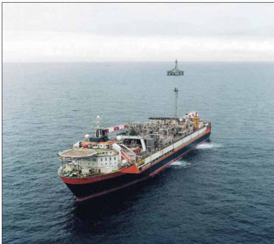
Statoil developed Norne with a production and storage vessel that possesses a processing plant on deck and storage tanks for stabilized oil (photo from Statoil).
