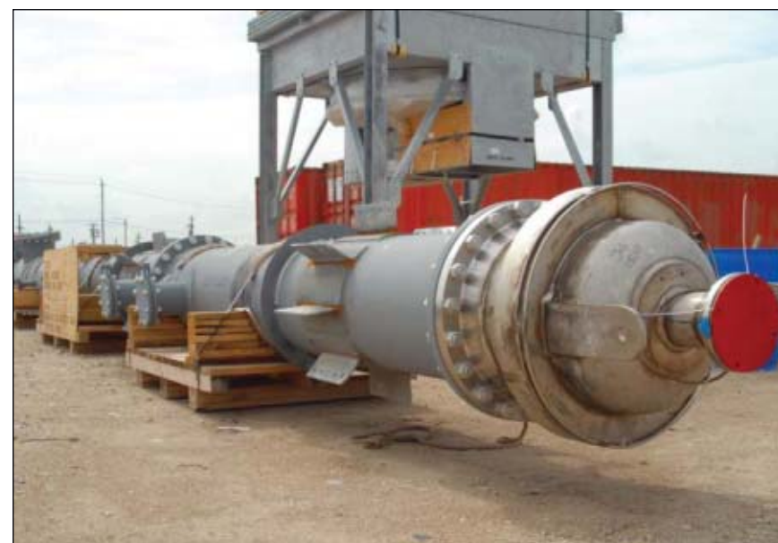
The sour water stripper column, left, and various modules, right, await transport to the Kurdistan region of Iraq.
